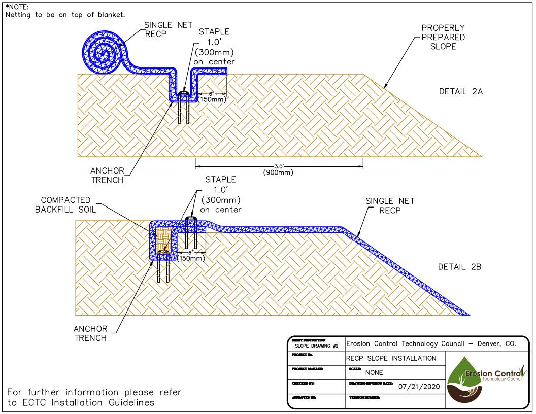
\*NOTE: Netting to be on top of blanket. SINGLE NET **PROPERLY STAPLE** RECP PREPARED 1.0' SLOPE (300mm)on center XXXXXXX XXXXX DETAIL 2A (150mm) 3.0'— (900mm) ANCHOR STAPLE **TRENCH** 1.0' (300mm)COMPACTED SINGLE NET BACKFILL SOIL on center **RECP** (150mm) DETAIL 2B ANCHOR **TRENCH**
