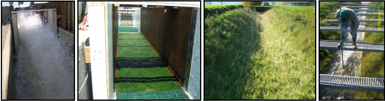
Figure 3. Research being conducted on TRMs to establish performance/permissible design values (Images in order from left to right. High shear stress flow over reinforced vegetation in vertical walled flume, reinforced vegetation after flow, reinforced vegetation in trapezoidal channel before flow, measuring velocity during flow over reinforced vegetation)
