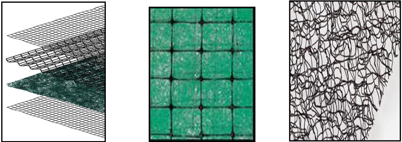
Figure 5. TRMs are constructed from a variety of materials that impart different performance characteristics, however, the one thing in common among all TRMs is the presence of a permanent three-dimensional structure for effective vegetation reinforcement.
